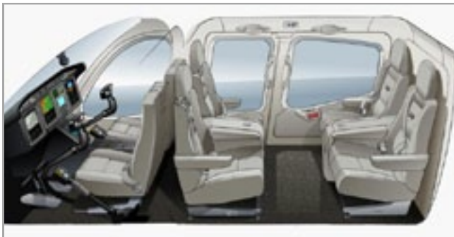
Four place club seating with two 21.5" seats separated by a center console in each row
