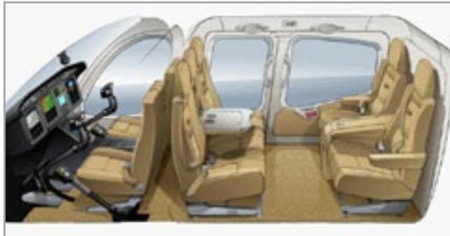
Five place club seating with a row of two 21.5" seats separated by a center console facing a row of three 18.5" seats with a center seat fold-down table
